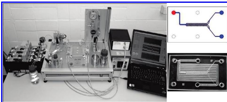
Figure 1. Multipurpose microreaction setup used in the present study, and the X-mixer from the Little Things Factory. 29
